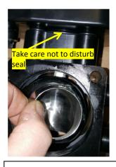
Step 6: Remove the ball. <u>Take</u> note of the position of the ball in the valve
