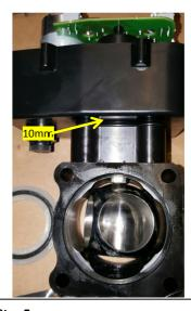
Step5: Lift the motor drive from the housing 10mm to allow the drive to disengage from the ball
