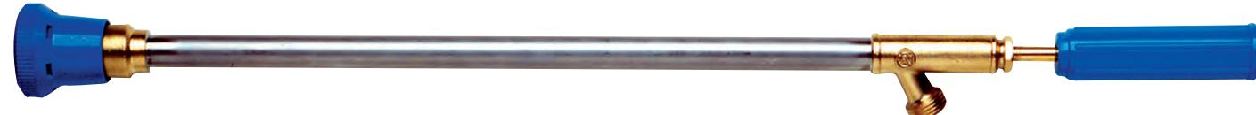
*Stainless steel spray gun, fitted with nozzle by request (see chart) and pipe fitting Ø8 - Ø10 - Ø13 (to be specified). The spray angle adjustment, from hollow cone to solid stream and shut/off is obtained by rotating the handle.*
