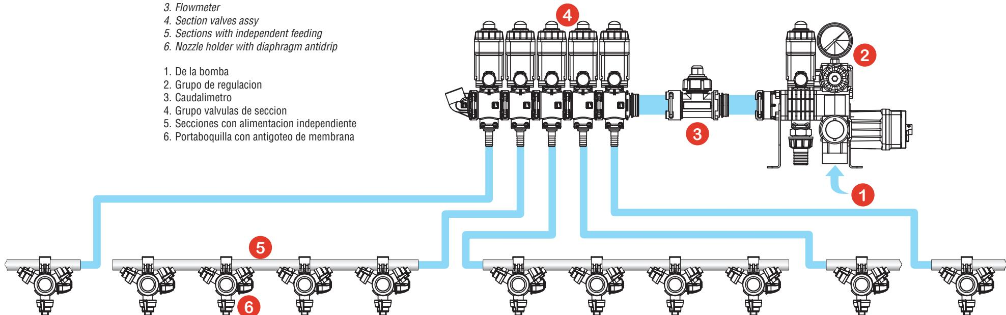
**ESEMPIO DI CONFIGURAZIONE BARRA A FLUSSO CONTINUO - EXAMPLE OF CONTINUOUS FLOW BOOM CONFIGURATION
