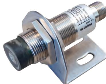
**WSA antenna is a GPS speed sensor, which allows to measure the feed speed of the agricultural machine during the work phases. It can be mounted as an alternative to the sensor on the wheel, simplifying installation and reducing the possible causes of failure of the traditional speed sensor.**
