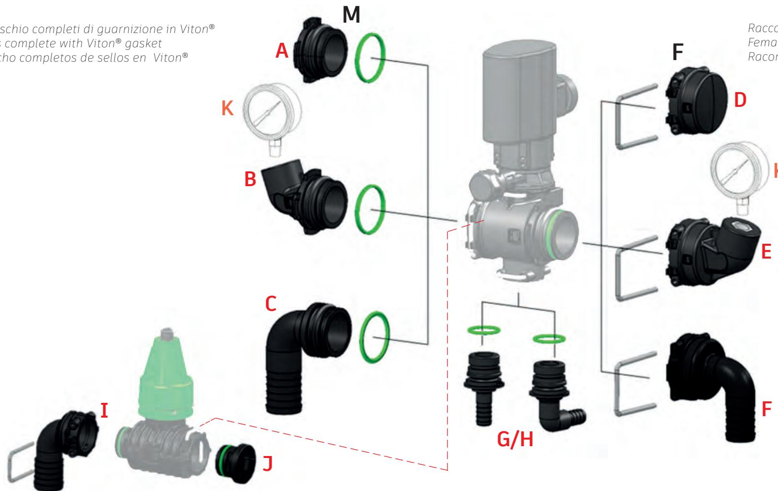
*The composition of Series 5 control units concludes with selection of the completion fittings, to be chosen in accordance with the agricultural machinery connection needs.*
